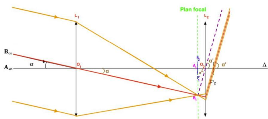
$$G = \frac{\alpha'}{\alpha} = \frac{\frac{A_1 B_1}{f'_2}}{\frac{A_1 B_1}{f'_1}} = \frac{A_1 B_1}{f'_2} \times \frac{f'_1}{A_1 B_1} = \frac{f'_1}{f'_2}$$
